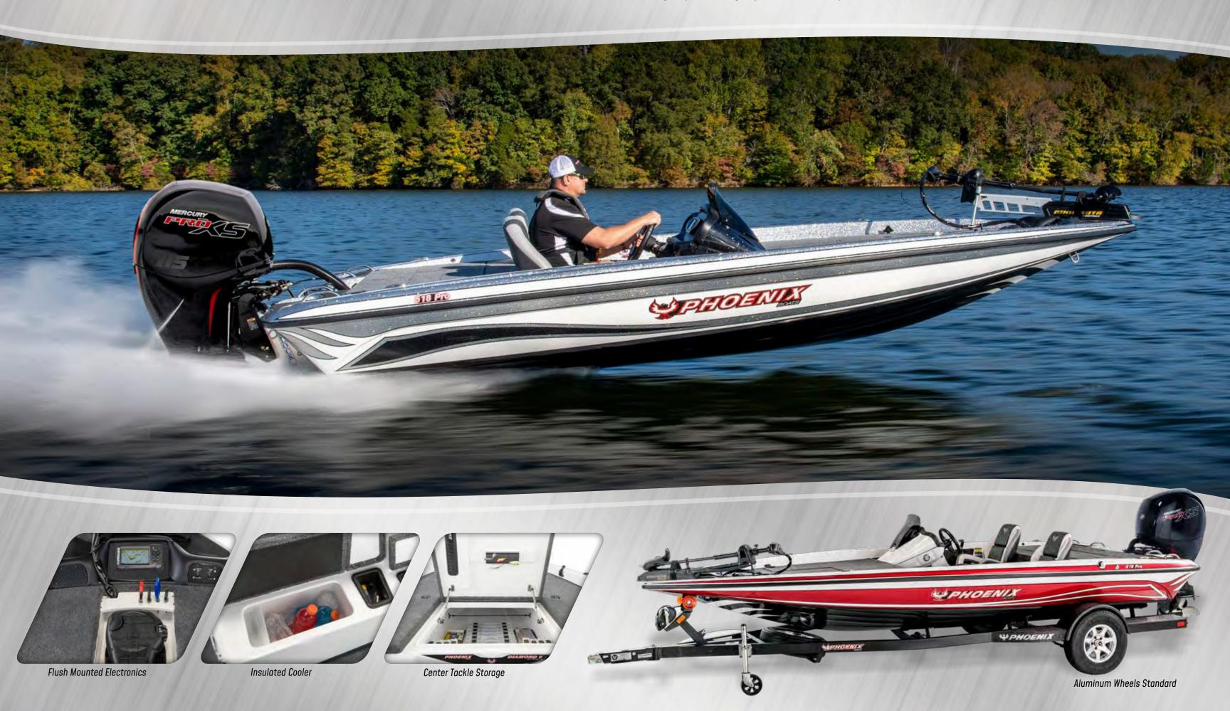
FUEL CAPACITY **24 GAL** MAX HP **II5 HP** LENGTH **18'6"** APPROXIMATE LENGTH ON TRAILER 21'11"\* W/ TONGUE FOLDED AND MERCURY MOTOR IN DOWN POSITION WEIGHT (APPROX) 1500 LBS BEAM **94**" LIVEWELL CAP 34 GAL. \* LENGTH MAY VARY WITH OPTIONS
